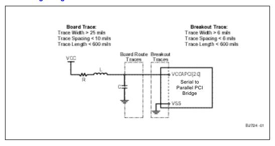
*Note:* Three of these PCI filter circuits must be placed on the system board, one for each of the **VCCAPCI[2:0]** pins on the 41110.
